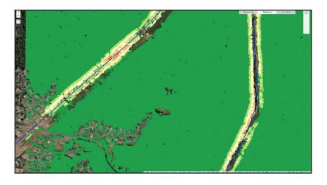
Figure 2: From Lidar data risk of arcing is interpolated. 3D viewing provides context and verification.
